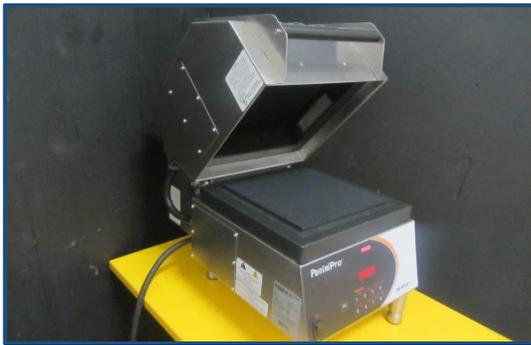
USING A NON-ABRASIVE CLOTH WITH A MILD DETERGENT & WARM WATER, WIPE DOWN THE ENTIRE OUTSIDE OF THE PRESS.
