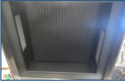
USING A NON-ABRASIVE CLOTH WITH A MILD DETERGENT & WARM WATER, WIPE DOWN THE ENTIRE UPPER COOKING SURFACE, THIS INCLUDES THE (2) WAVE GUIDE COVERS AND SURROUNDING SURFACES. ENSURE THAT ALL RESIDUAL FOOD AND DEBRIS ARE WIPED AWAY.
