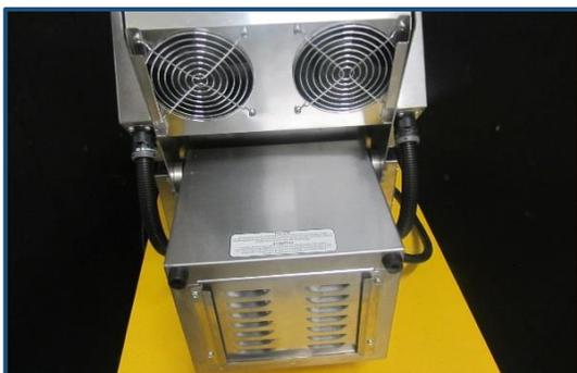
USING A NON-ABRASIVE CLOTH & WARM WATER WIPE DOWN THE AREAS LOCATED BEHIND THE FILTERS. ENSURE THAT NEITHER OF THE FAN COVERS OR THE VENTS ARE BLOCKED BY DEBRIS - IT IS ESSENTIAL TO CORRECT OPERATION THEY ARE FREE & CLEAR.
