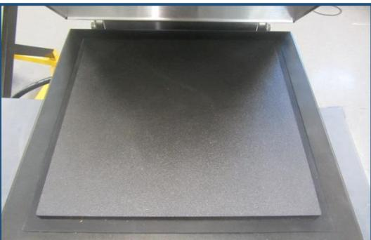
USING A NON-ABRASIVE CLOTH WITH A MILD DETERGENT & WARM WATER, WIPE DOWN THE ENTIRE LOWER COOKING SURFACE, THIS INCLUDES THE AREA SURROUNDING THE HEATER PLATE. ENSURE THAT ALL RESIDUAL FOOD AND DEBRIS ARE WIPED AWAY.
