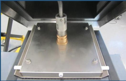
USING A NON-ABRASIVE CLOTH WITH A MILD DETERGENT & WARM WATER, WIPE DOWN THE TOP SIDE OF THE UPPER HEATER PLATE ASSEMBLY. ENSURE THAT ALL RESIDUAL FOOD AND DEBRIS ARE WIPED AWAY.
