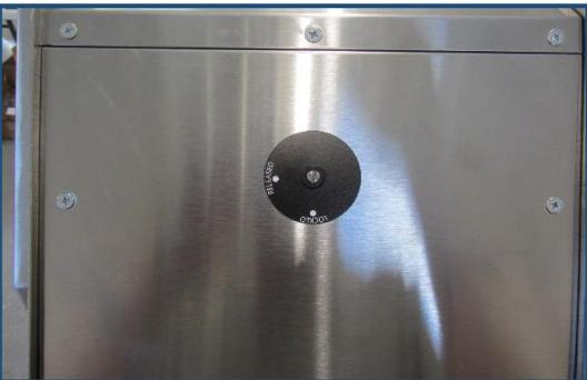
RE-INSTALL TOP HEATER PLATE ASSEMBLY INTO THE TOP CAVITY. INSERT THE POST INTO THE BUSHING IN THE TOP CAVITY AND TURN THE RELEASE SHAFT TO THE LOCKED POSITION.
