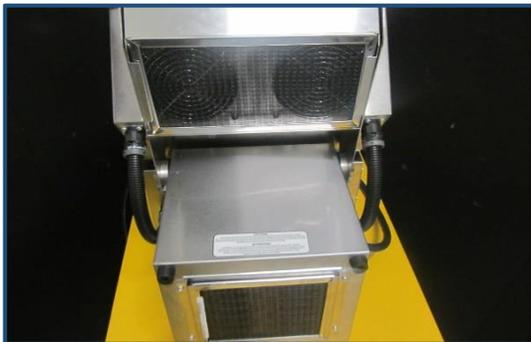
REMOVE BOTH AIR FILTERS LOCATED ON THE REAR OF THE PRESS.
