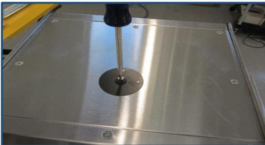
AT THE END OF EACH DAY, DROP THE UPPER HEATER PLATE ASSEMBLY FOR CLEANING. THIS CAN BE DONE BY TURNING THE RELEASE SHAFT ON TOP OF THE PRESS TO THE RELEASED POSITION. A TOWEL SHOULD BE PLACED ON THE LOWER HEATER PLATE BEFORE THE UPPER HEATER PLATE IS RELEASED TO PROHIBIT DAMAGE TO THE TEFLON COATING.
